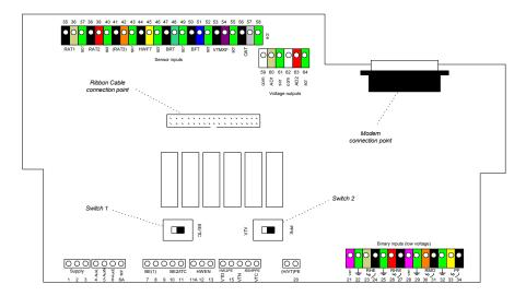
Power Supply Unit (PSU) board incorporating output relays, terminals and 25 pin, RS232 port connection for a modem.
